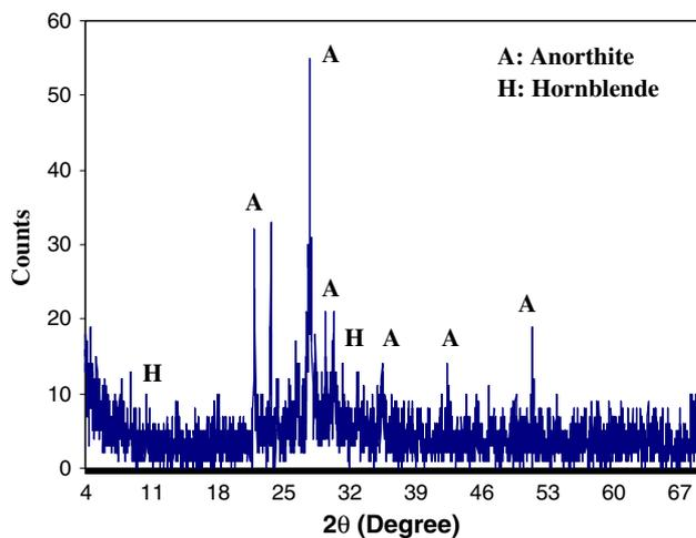
**Fig. 13** X-ray diffraction patterns of mix IP2 cured at 85 °C for 20 h after 7 days of pre-curing
