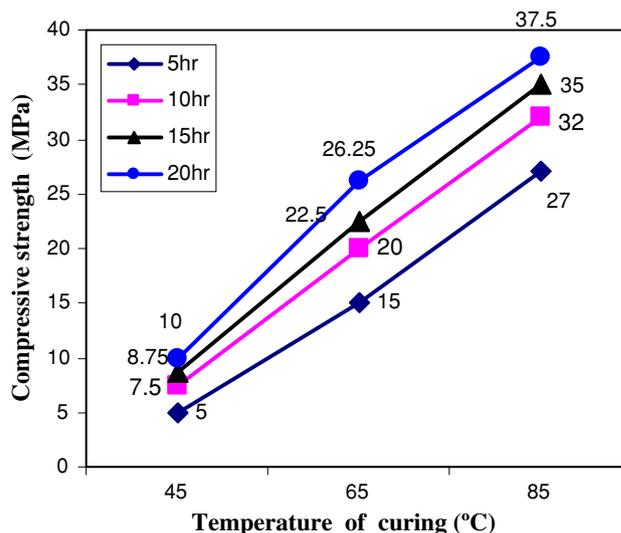
**Fig. 6** Effects of temperature and time of hydrothermal curing on compressive strength development after 1 day of precuring for mix IP2
