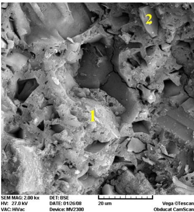
**Fig. 19** SEM image of mix IP2 cured at temperature of 210 °C for 30 h after 7 days of precuring (magnification: 2000×)
