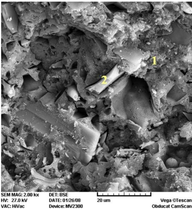
**Fig. 18** SEM image of mix IP2 cured at temperature of 125 °C for 20 h after 7 days of precuring (magnification: 2000×)
