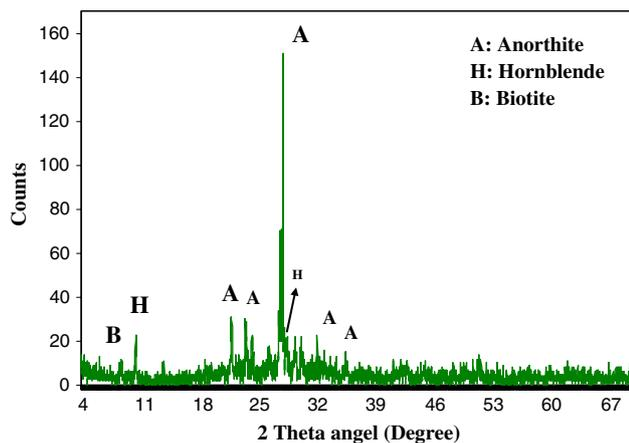
**Fig. 1** X-ray diffraction pattern of pozzolan
