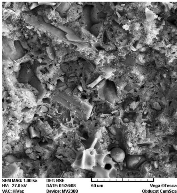
**Fig. 22** SEM image of mix IP2 cured at temperature of 125 °C for 20 h after 7 days of precuring (magnification: 1000×)
