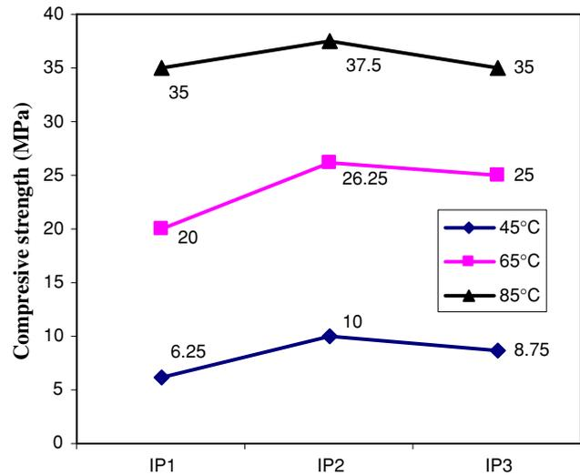
**Fig. 10** Effects of different temperatures of hydrothermal curing for a period of 20 h on compressive strength development after 1 day of precuring for different mixes
