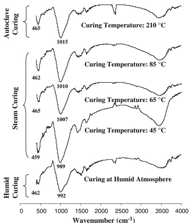
**Fig. 15** FTIR spectra of mix IP2 cured under different curing conditions
