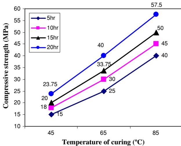
**Fig. 7** Effects of temperature and time of hydrothermal curing on compressive strength development after 7 days of precuring for mix IP2
