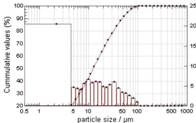
**Fig. 3** Particle size distribution of ground pozzolan
