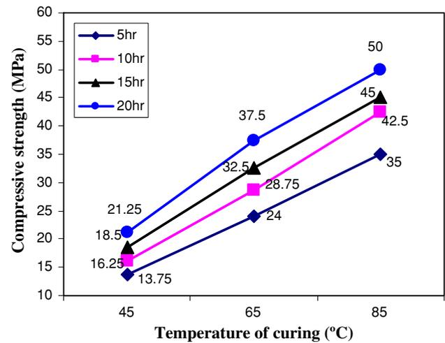
**Fig. 9** Effects of temperature and time of hydrothermal curing on compressive strength development after 7 days of precuring for mix IP3
