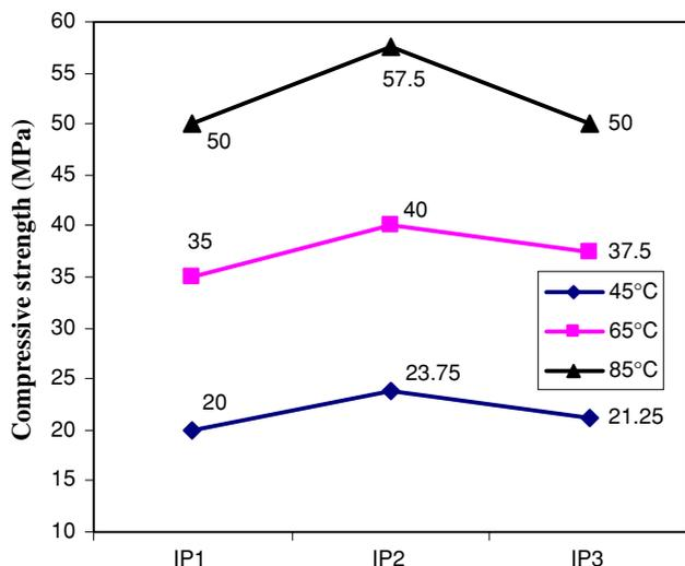
**Fig. 11** Effects of different temperatures of hydrothermal curing for a period of 20 h on compressive strength development after 7 days of pre-curing for different mixes
