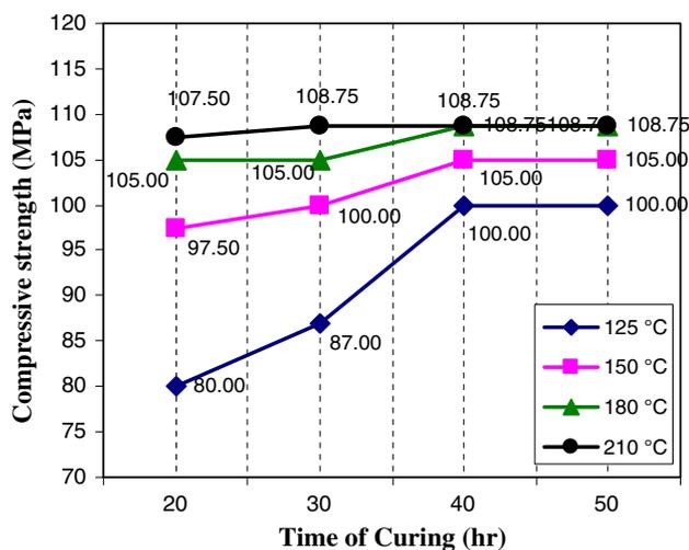
**Fig. 12** Effects of higher times and temperatures of autoclave curing on compressive strength development after 7 days of pre-curing for mix IP2
