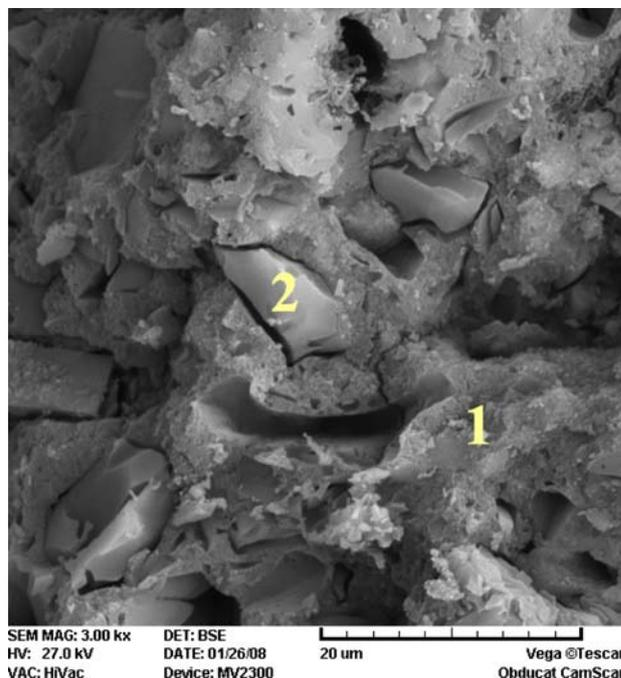
**Fig. 17** SEM image of mix IP2 cured at temperature of  $85\text{ °C}$  for 20 h after 7 days of precuring (magnification:  $3000\times$ )
