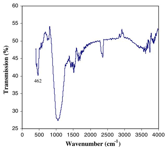
**Fig. 2** FTIR spectrum of pozzolan
