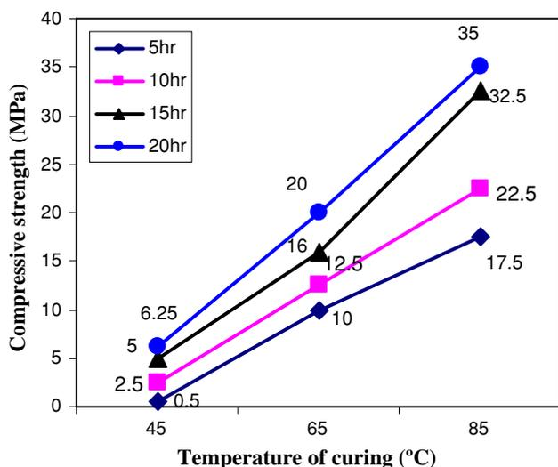
**Fig. 4** Effects of temperature and time of hydrothermal curing on compressive strength development after 1 day of precuring for mix IP1
