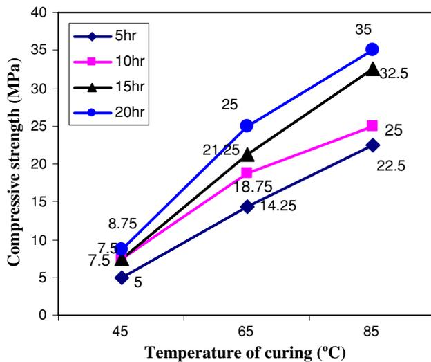
**Fig. 8** Effects of temperature and time of hydrothermal curing on compressive strength development after 1 day of precuring for mix IP3
