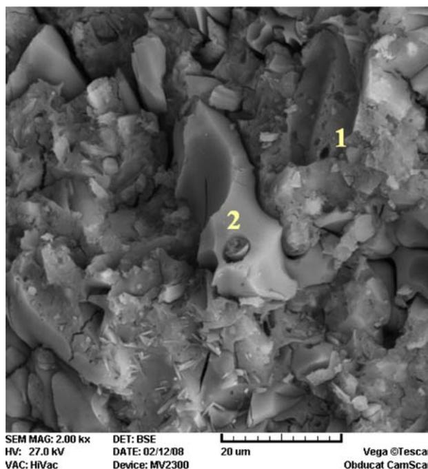
**Fig. 16** SEM image of mix IP2 cured for 28 days at more than 95% relative humidity at room temperature (magnification:  $2000\times$ )
