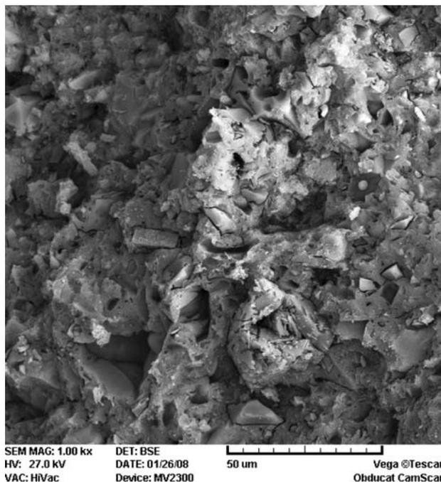
**Fig. 21** SEM image of mix IP2 cured at temperature of 85 °C for 20 h after 7 days of precuring (magnification: 1000×)
