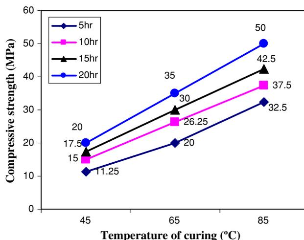
**Fig. 5** Effects of temperature and time of hydrothermal curing on compressive strength development after 7 days of precuring for mix IP1
