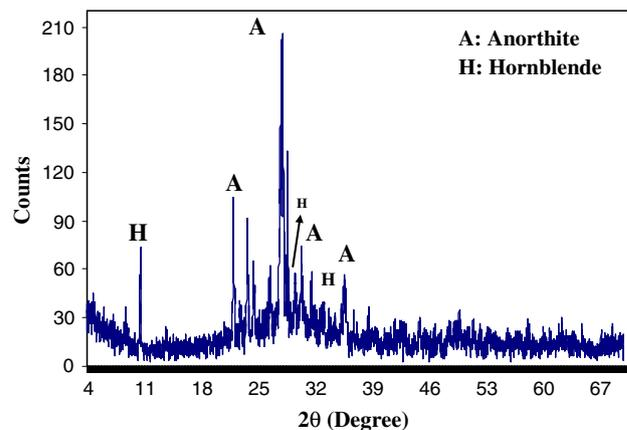
**Fig. 14** X-ray diffraction patterns of mix IP2 cured at 125 °C for 20 h after 7 days of pre-curing
